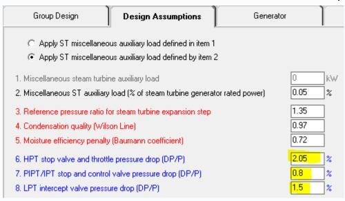
Required to correctly simulate the LP bowl pressure
